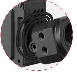
6. Wrap the connection cable between the O3 Air Unit and the camera three times. Then, place the camera between the two camera damping silicone pieces and secure it with four M2\*6mm (hex socket button head) screws.
