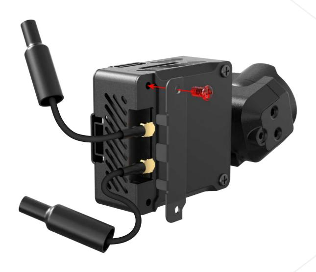
2. Install the provided antenna into the corresponding interface and secure the antenna cover with an original M1.6\*8 Phillips screw.
