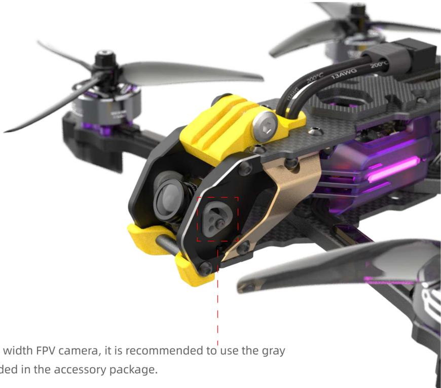
When using a 19mm width FPV camera, it is recommended to use the gray camera mount included in the accessory package.
