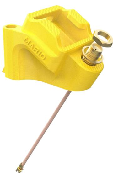
3. Install the SMA pigtail cable.
