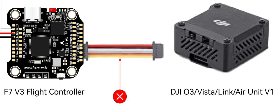
Do NOT connect this wire to assure the external SBUS receiver work properly!
