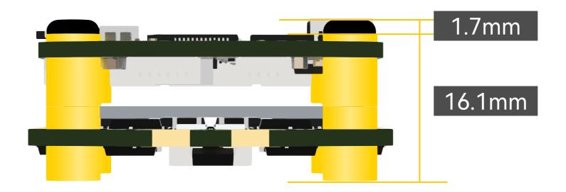
Please ensure that the Stack is installed in the standard manner, with the flight controller (FC) on top and the electronic speed controller (ESC) on the bottom. Any damage resulting from improper installation is not covered under our warranty.
